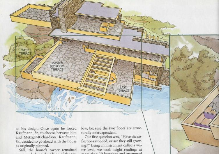
Still, the house's owner remained concerned about the tilting of the terraces, so he commissioned a surveyor to measure the deflections on a regular basis by recording the elevations of the tops of the parapet walls. This was done from 1941 until 1955, when Kaufmann, Sr., died. In 1963 Kaufmann, jr., presented the house to the Western Pennsylvania Conservancy. Between 1955 and the time our firm was retained in 1995, only one or two random measurements of the terraces' deflections were recorded.
